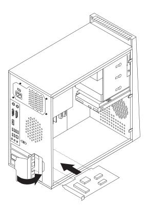
Figure 8. Closing the adapter card latch
